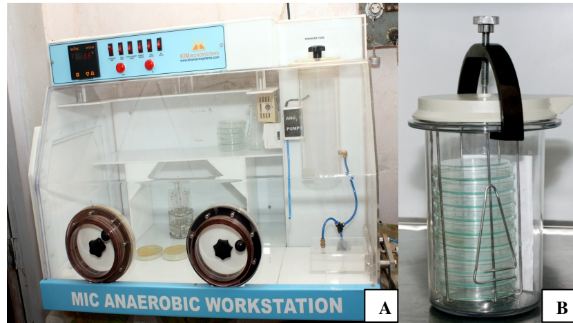
Fig. 1. Equipments for the maintenance of anaerobic condition. A. Anaerobic workstation; B. Anaerobic jar
